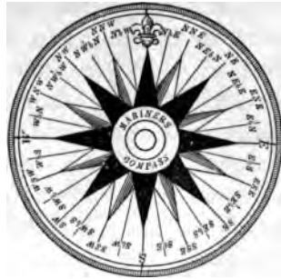
FIG. 93. The Mariner's Compass. The needle always points to the north, and therefore sailors can steer by it.
